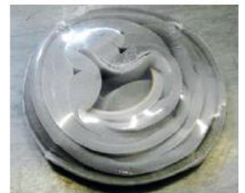
Pre-compressed tape packed up in plain lamination sheet after accelerated storage / Institut OFI, Vienna
