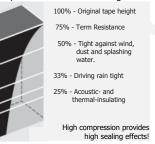
The edition of compriband combi, i.e. the closed Comprilen should be pressed against a smooth surface (metal etc.) in order to achieve the optimal sealing effect. Thus, the Comprilen ends with the metal, however, the open-celled Compriband-A can be stuck on rough and smooth surfaces.
